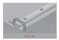
Fasten bolts temporarily and push a master rail toward the datum plane using a C-vise. Fasten the bolts sequentially at the pre scribed torque.
